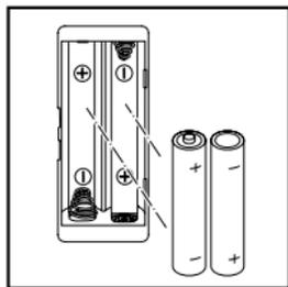
In case of a power failure, the appliance relies on battery backup. For this purpose, the appliance uses two batteries (AAA). The appliance remembers the time, but does not display it.
